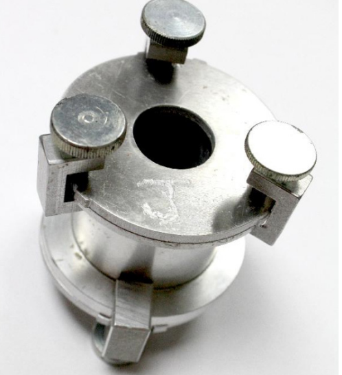
Figure 1. Standard Paddington Cup. The film dressing is clamped across the open annular plate, which provides a 10 cm² area for evaporation. A volume of 20 ml is used.
