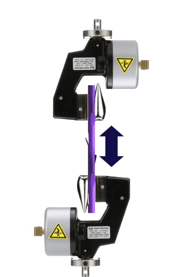
Figure 2. Straight Pull Force test method
