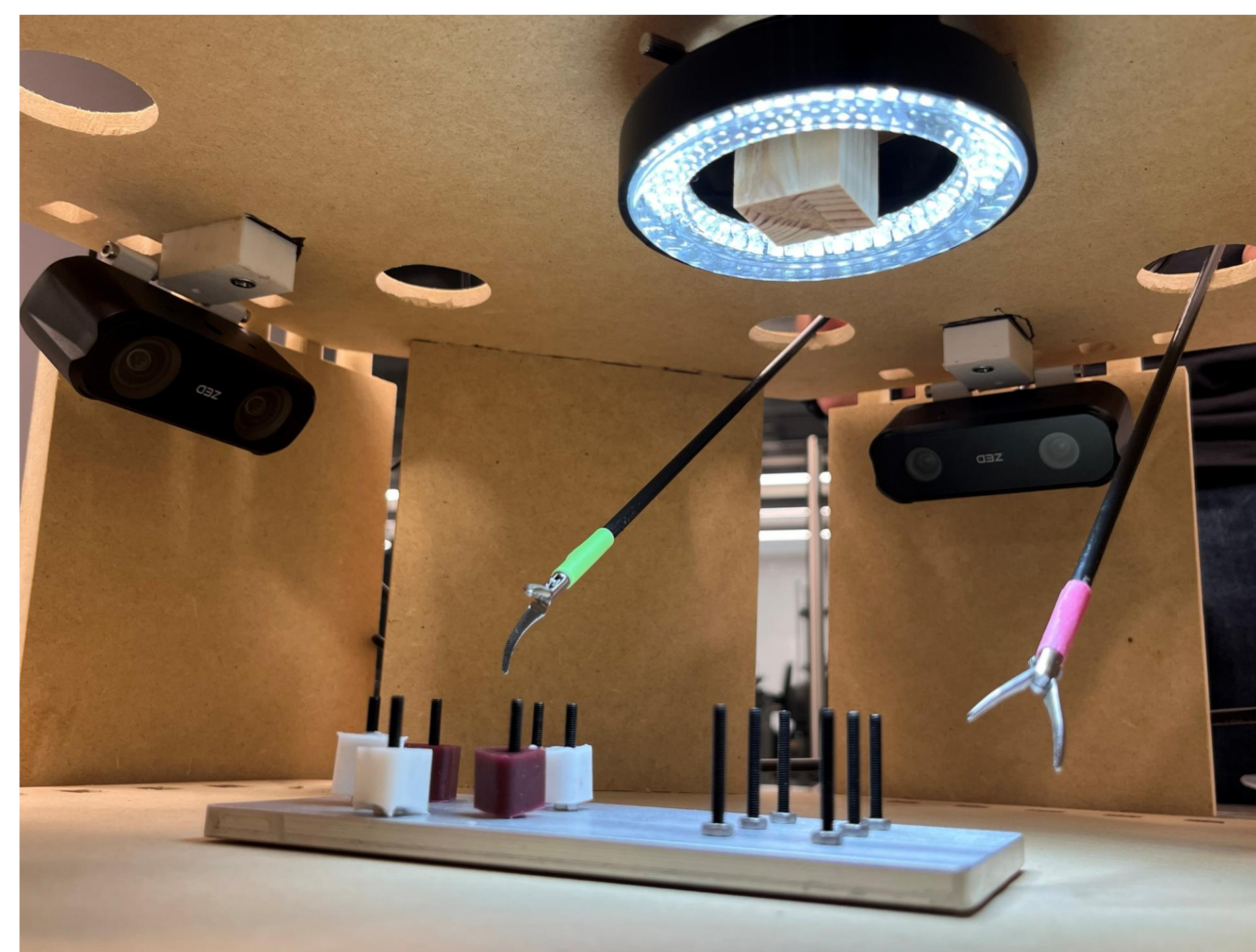
Figure 1. a) Workflow overview of the LapTrackr system, b) Pilot testing results from 2 users, c) Annotated user view and depth map of instruments inside the training enclosure., D) user software interface of the system, E) interior of the LapTrackr enclosure showing the light source, dual camera setup and access ports for laparoscopic instruments.
