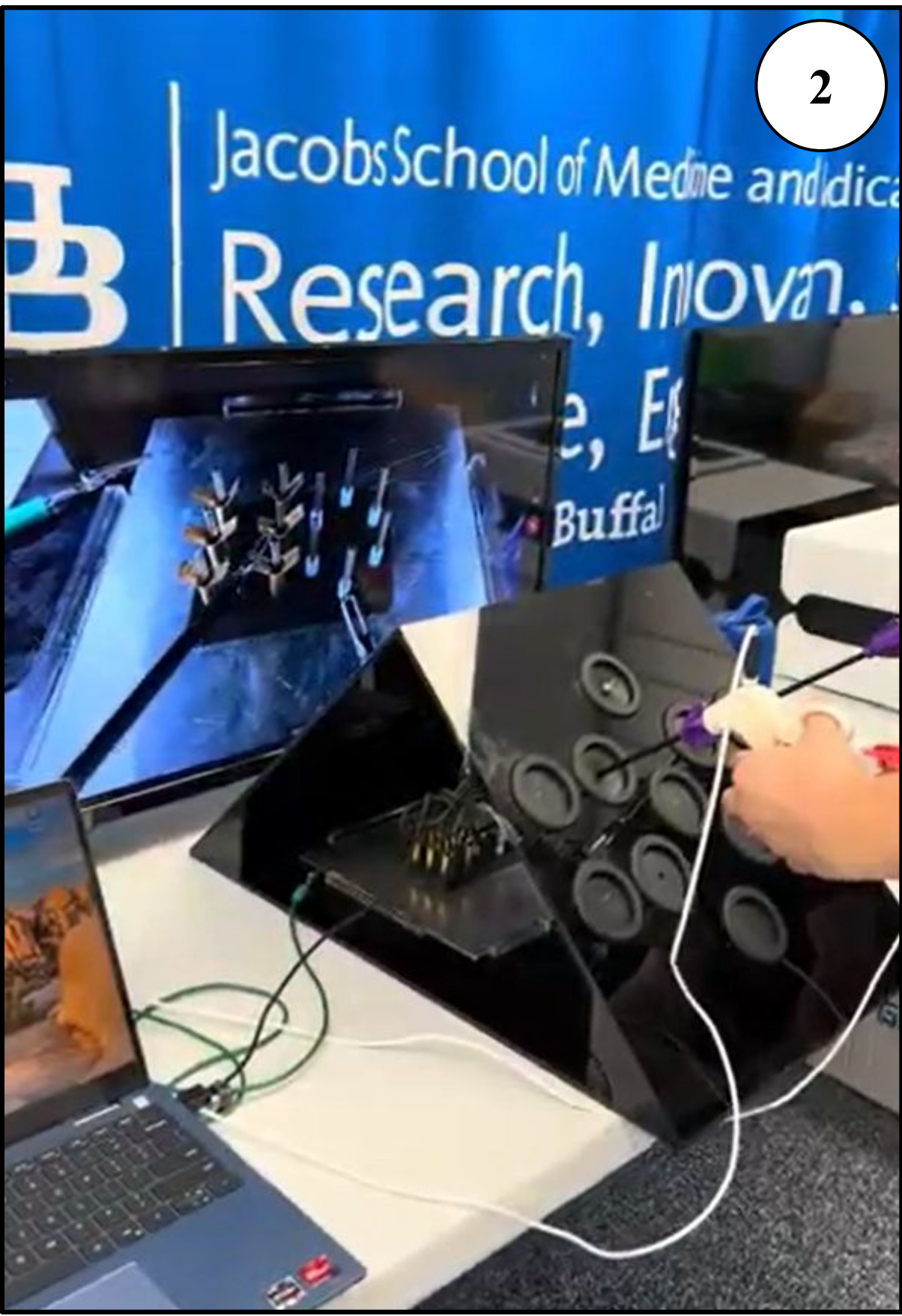
Figure 1: The acrylic tower (9 x 11.5 x 36 cm) stands on an acrylic base (15 x 25.3 x 23.5 cm) and houses all electronic components including: Arduino Uno, wiring, light, buzzer, and error counter. Two white instrument wires and a green metal plate wire connect to the simulator box. A black charging wire can be connected. Figure 2: The simulator box itself (57.5 x 30.5 x 29.5 cm) is an acrylic pyramid designed to simulate the abdomen. Rubber grommets are installed as trocars for instrument insertion.
