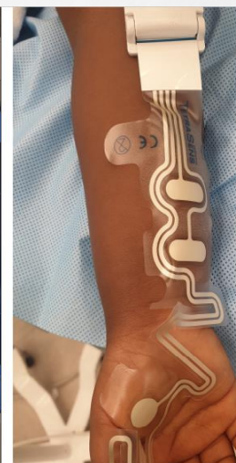
Figure 3: Recording electrodes (palmar surface) and stimulating electrodes (forearm) from pediatric sized sensor (TetraSens™)
