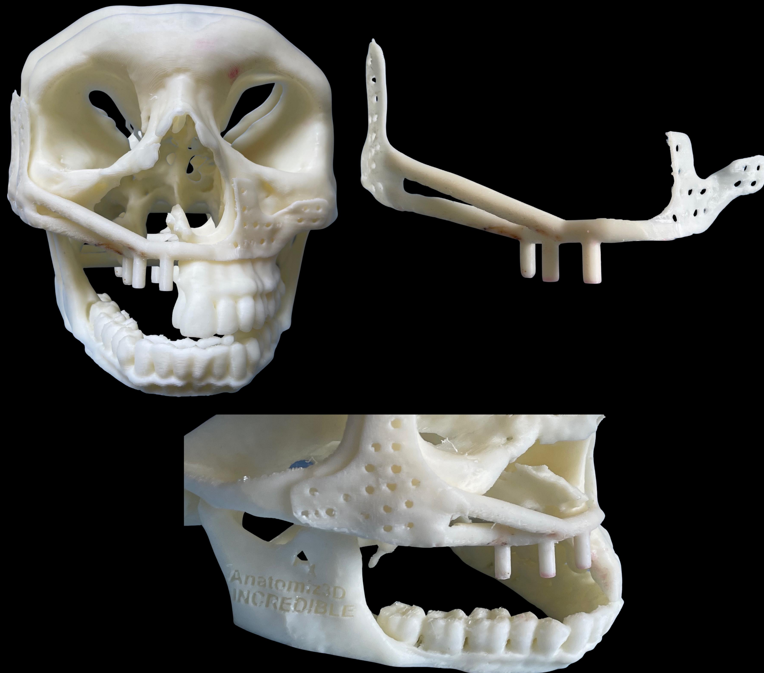
Stereolithographic Model with Planned Patient-Specific Implant Framework
