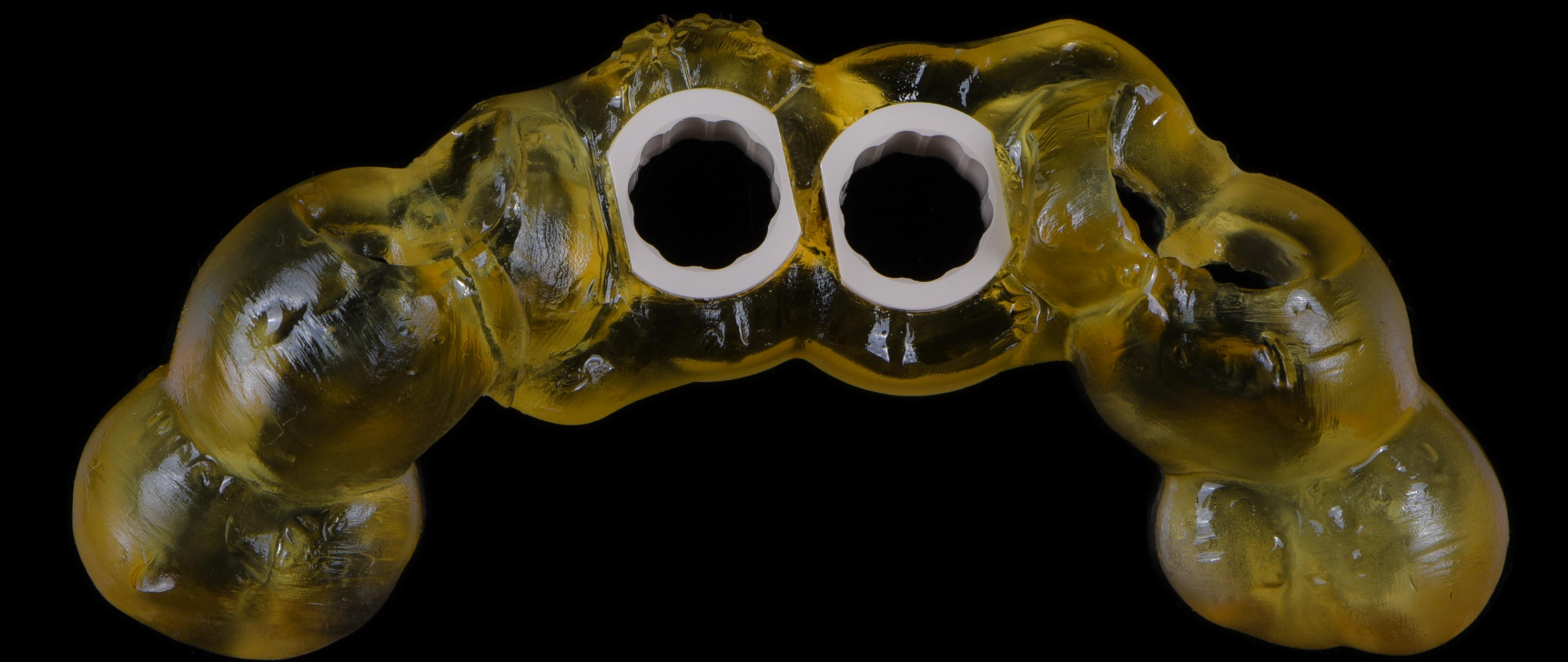
Additive manufactured s-CAIS
