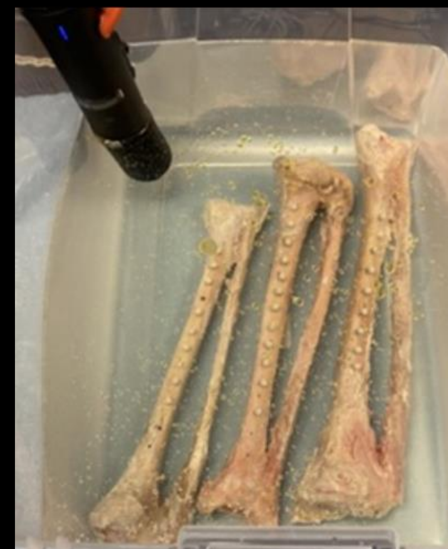
Figure 4: Three human cadaver tibias placed with cement zirconia crowns in saline water bath at 37 degrees Celsius.
