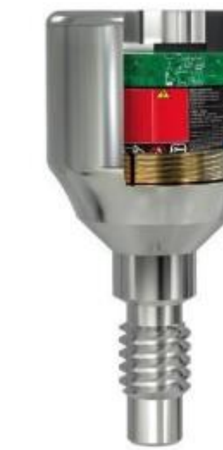
Figure.1 A cross-sectional view of the Miniaturized Electromagnetic Device (MED) healing abutment
