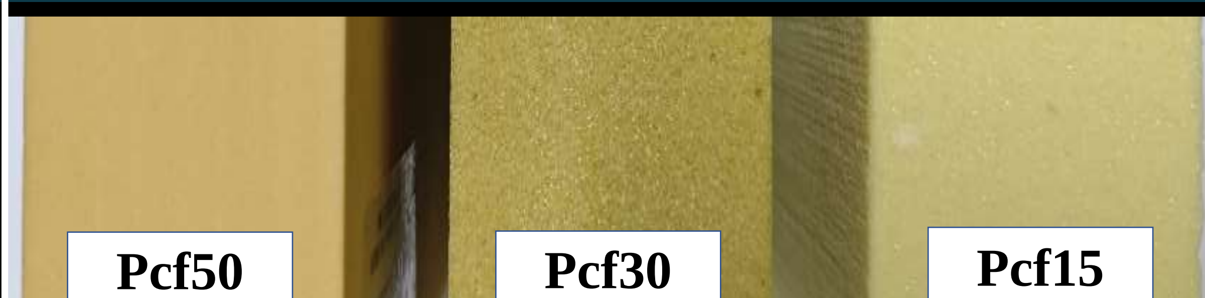
Artificial Bone Blocks of Different Densities
