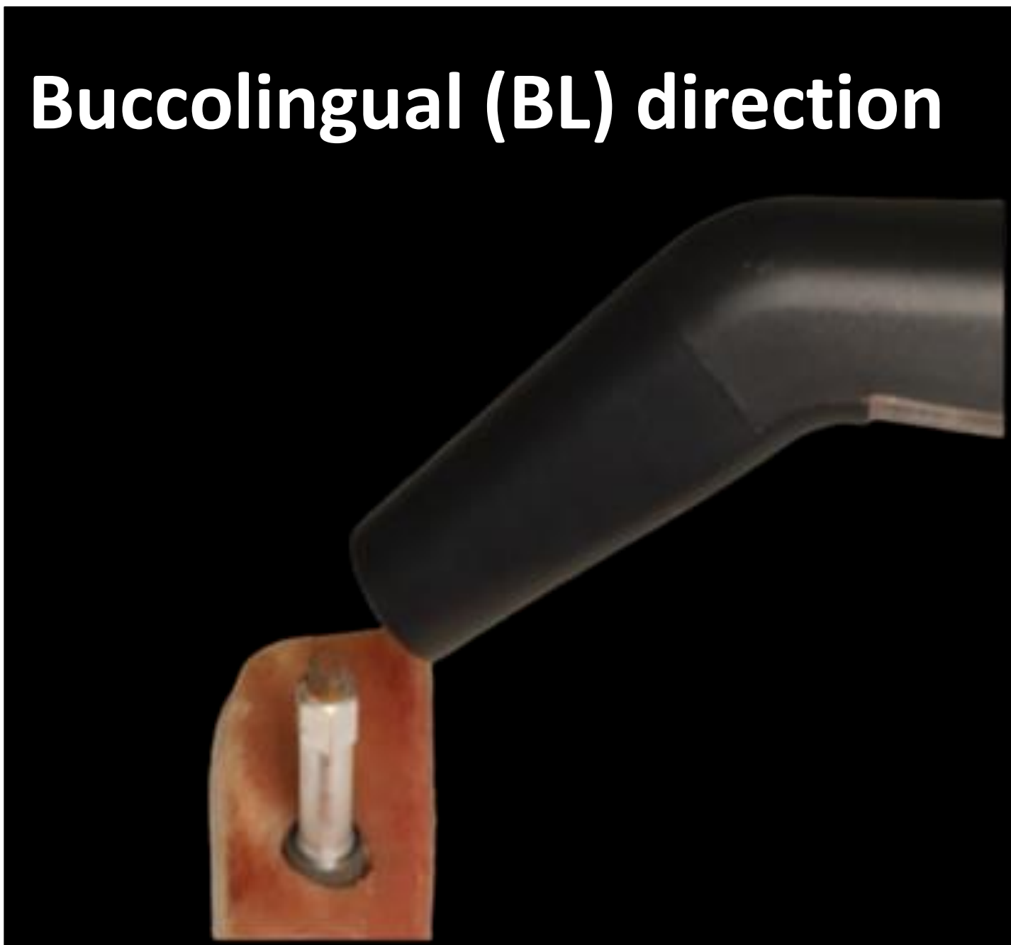
Fig.4: ISQ measurements were taken in both the mesiodistal (MD) and buccolingual (BL) directions for each implanted implant.
