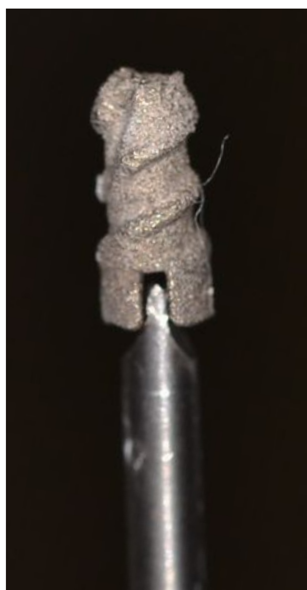
Fig 1. 2 x 4 mm implant produced by additive manufacturing process
