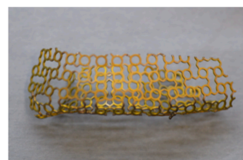
3D printed bone model and costumed Ti mesh.
