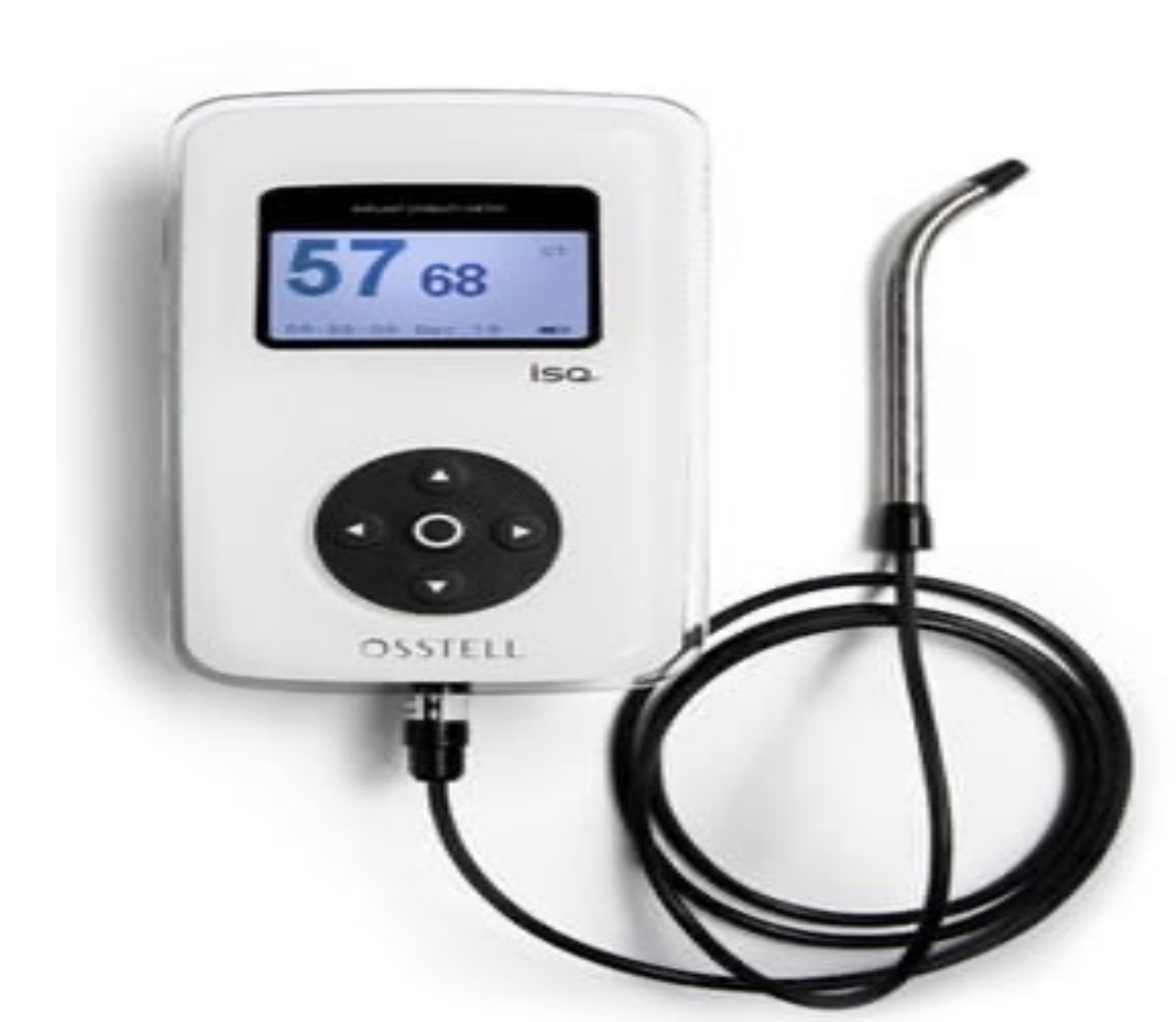
Figure 5: Osstell device for resonance frequency analysis (RFA)
