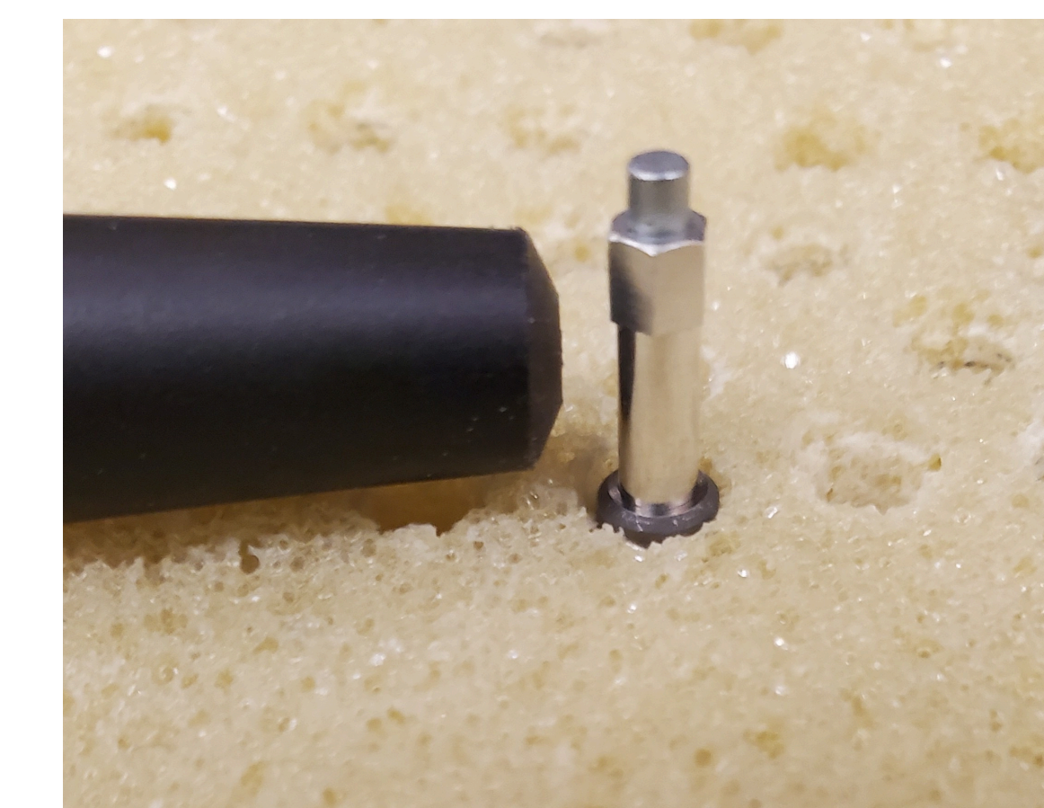
Figure 4: Implant with SmartPeg insert placed for implant stability measurement
