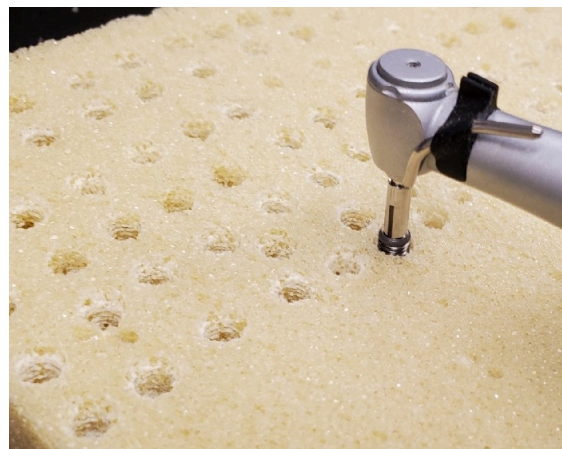
Figure 3: Implant placement in artificial, polyurethane, soft (type IV) bone
