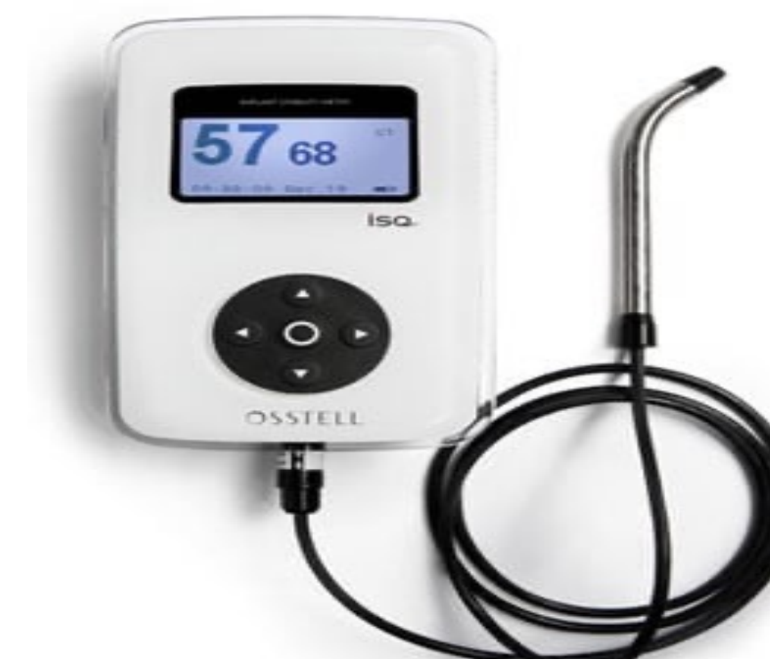
Figure 5: Osstell device for resonance frequency analysis (RFA)
