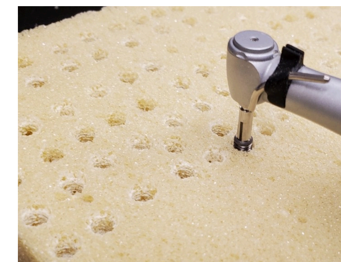
Figure 3: Implant placement in artificial, polyurethane, soft (type IV) bone
