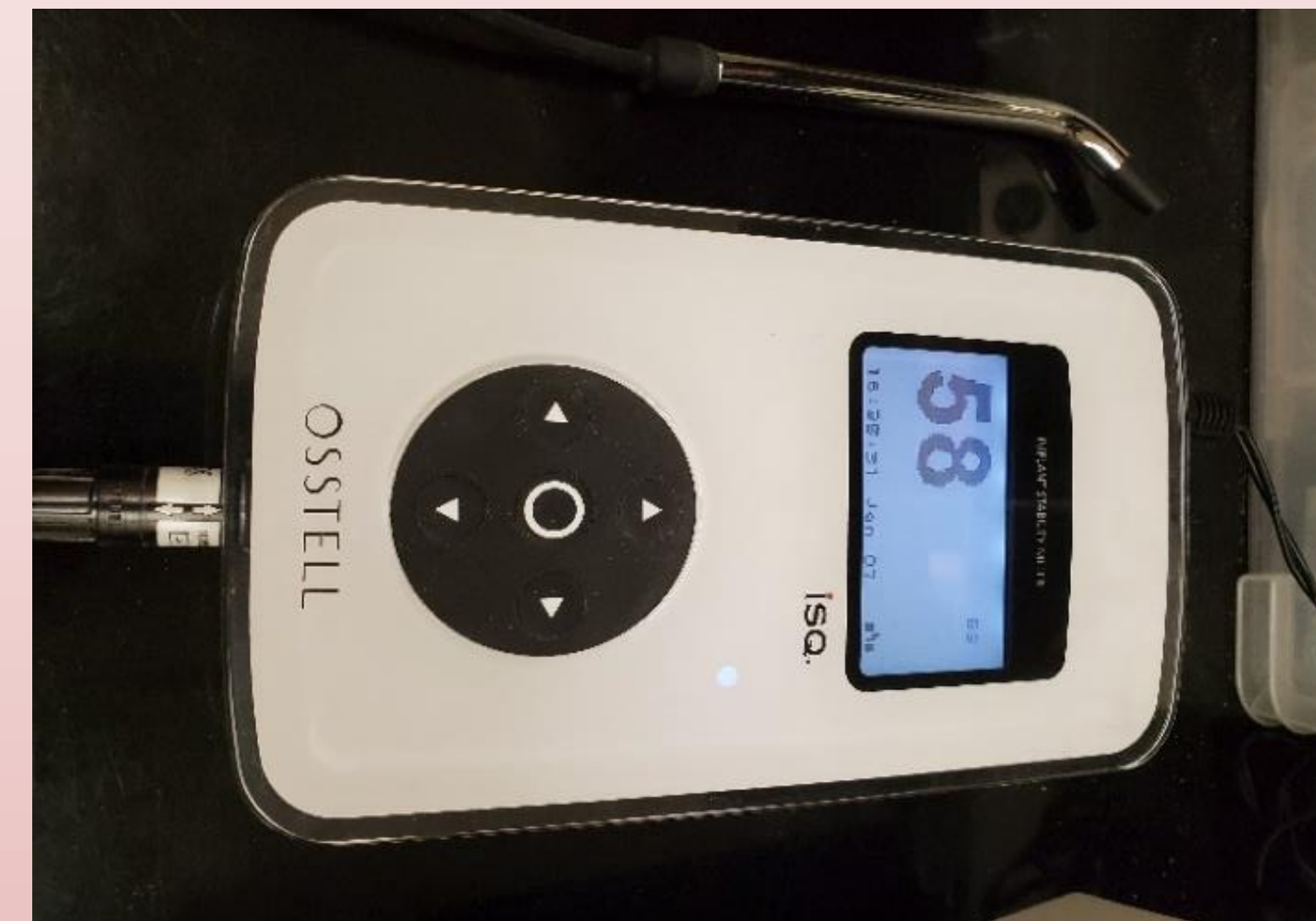
Fig. 1A. Ostell device used to evaluate PS of implants via RFA (Resonance Frequency Analysis)
