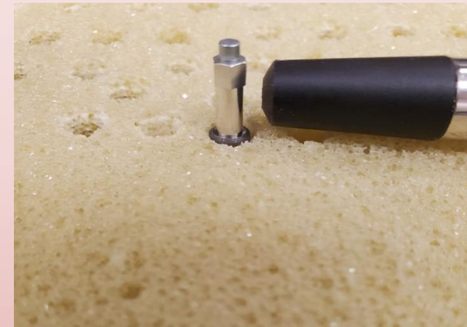
Fig. 1B. Short ImplantSwiss implants placement in Polyurethane soft bone resin block at bone level
