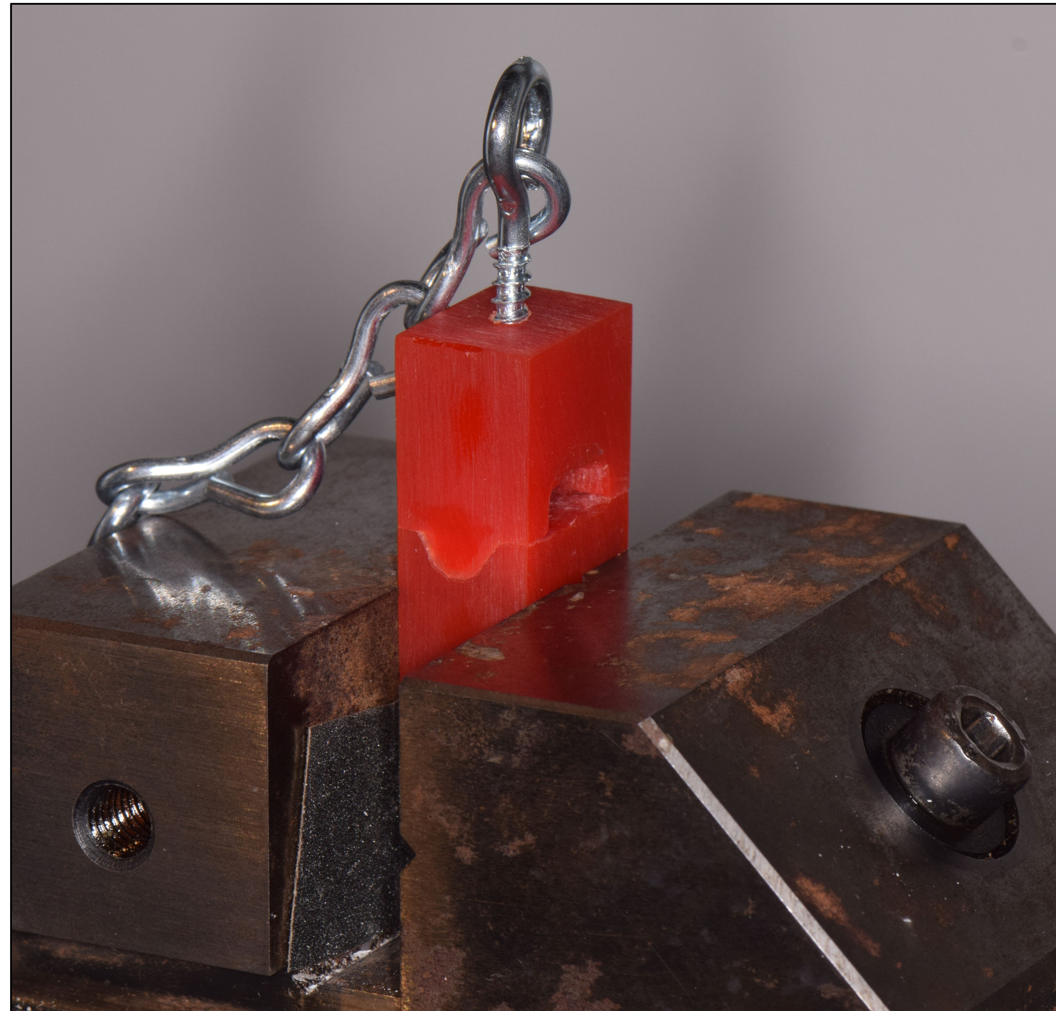
Figure 7. Attachment housings and overdenture abutment components were manually connected via the treated inserts. The pattern resin assembly was secured in a universal testing machine.
