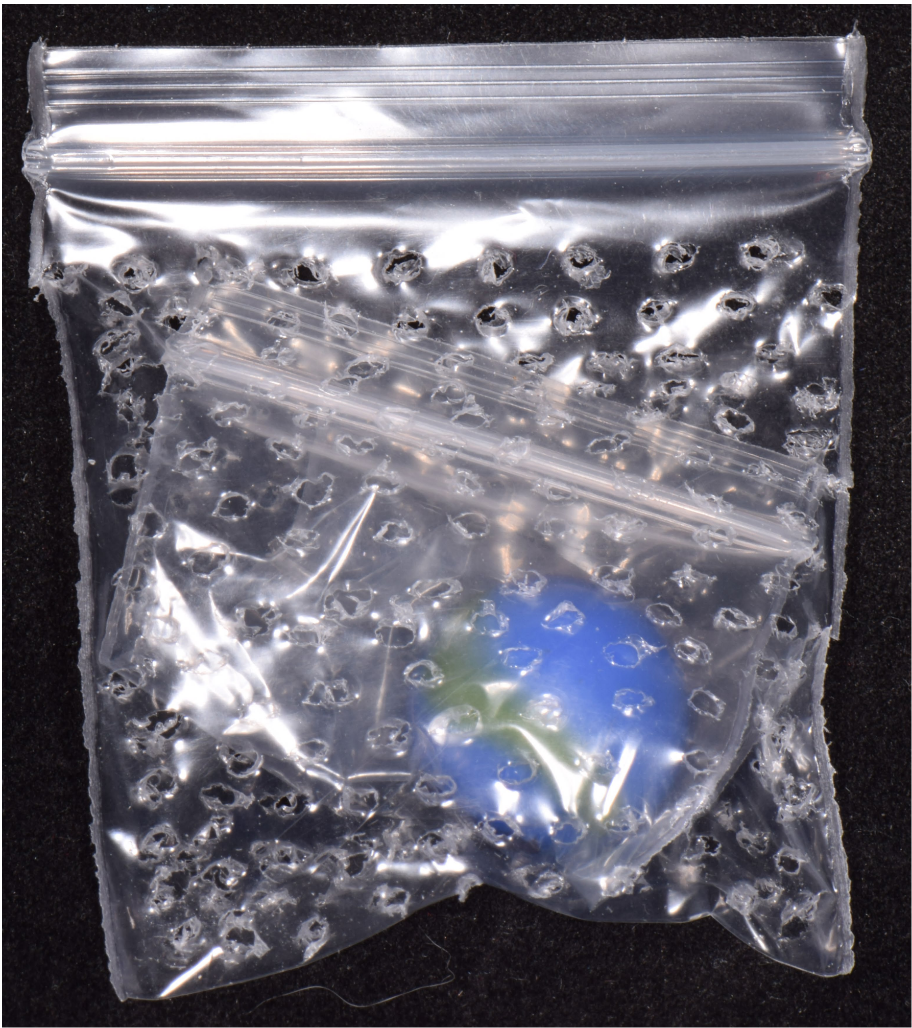
Figure 4. Groups of inserts (n=10) were randomly divided and placed into perforated plastic zip-lock bags with a separately-bagged marble.
