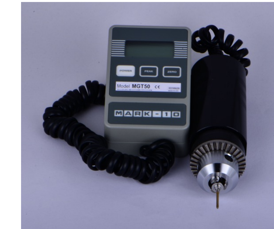
Fig. 4. A digital screw torque meter (MGT50; Mark-10) was used to measure screw torque values with decimal precision. The handle for the abutment screwdriver (UniGrip; Nobel Biocare AG) was mounted in the 3-jaw chuck of the digital screw torque meter. The abutment screw was tightened to 35 Ncm per manufacturer's recommendation twice, 10 minutes apart. Five minutes later, RTV was measured before CL and referred to as initial preload (IP). After CL, RTV was measured and referred to as final preload (FP).
