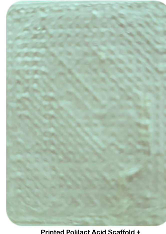
Printed Polilact Acid Scaffold + Collagen Membrane
