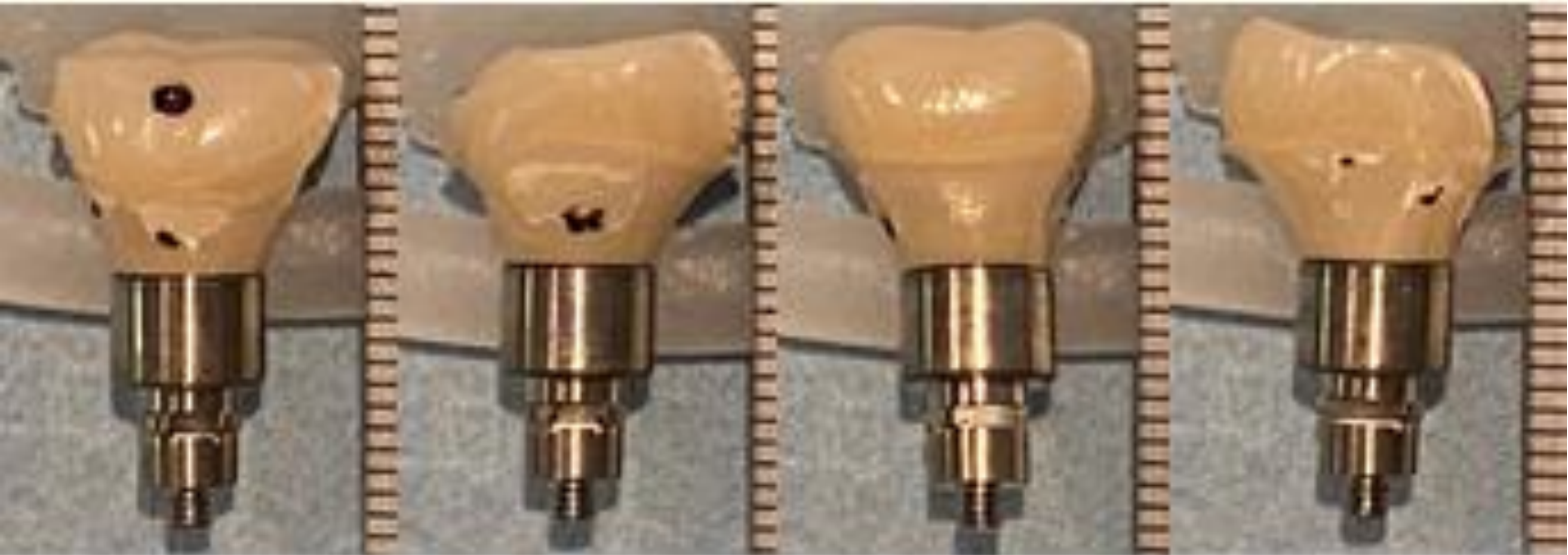
Fig 7: CMS with black dots showing cement travel beyond Buccal (B), Mesial (M), Lingual (L) and Distal (D) margins. Images placed beside mm ruler to measure cement travel distance.
