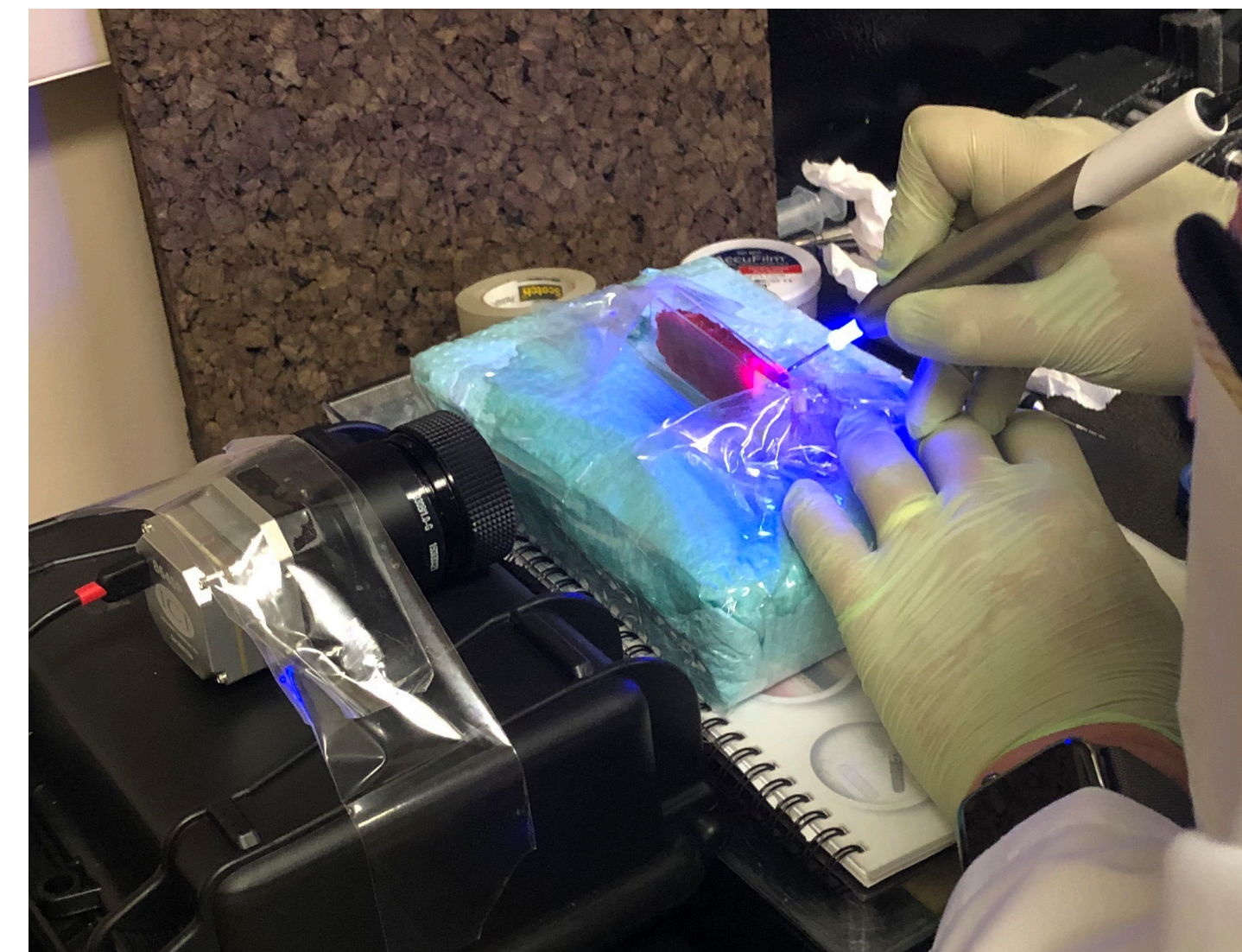
Fig. 1. Thermography camera is placed perpendicularly to the horizontal plane of the tissue, with 5mm thickness of bovine tissue placed between the glass slides. The sample is stabilized with clear tape to a flat surface, as the 980nm laser non-initiated glass fiber tip is incising the tissue in a horizontal manner.
