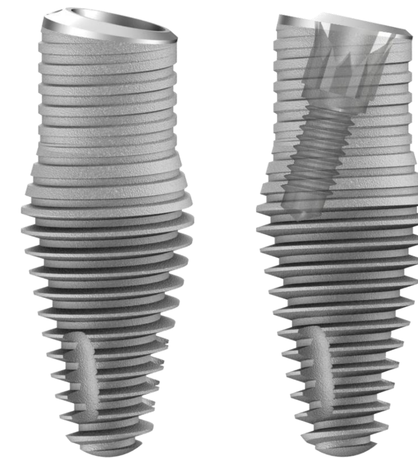
Fig.1 Hybrid design implant with 'body-shift' concept. Narrower cylindrical thread on coronal section and wider tapered thread on apical section. Angulated screw channel provides optimal prosthetic angulation.
