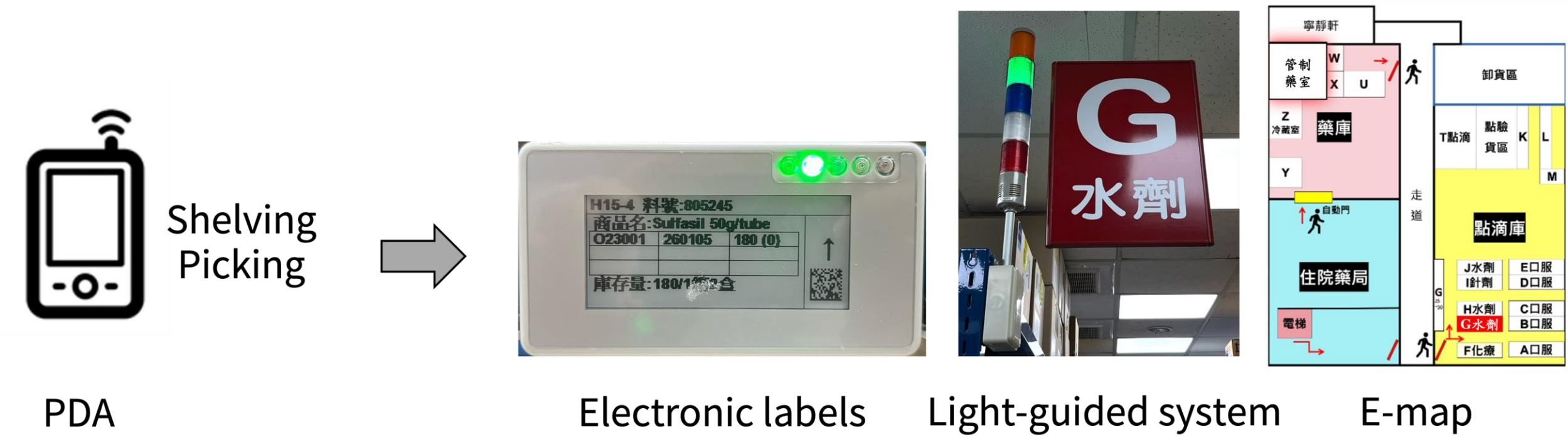
Fig. 5 When clerks perform shelving and picking, electronic labels and light-guided system will indicate the location of the medications.
