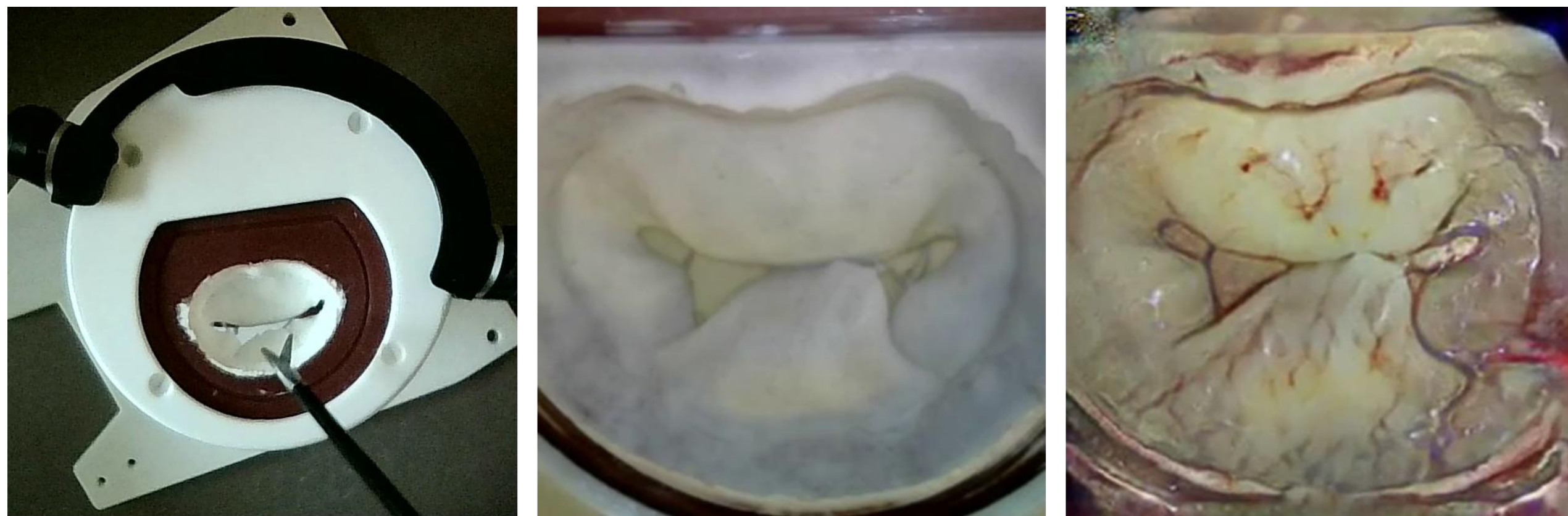
Figure 1: Silicone mitral valve phantom, endoscopic phantom view, and translated output demonstrating increased tissue coloration, blood-like appearance, and specular reflections.
