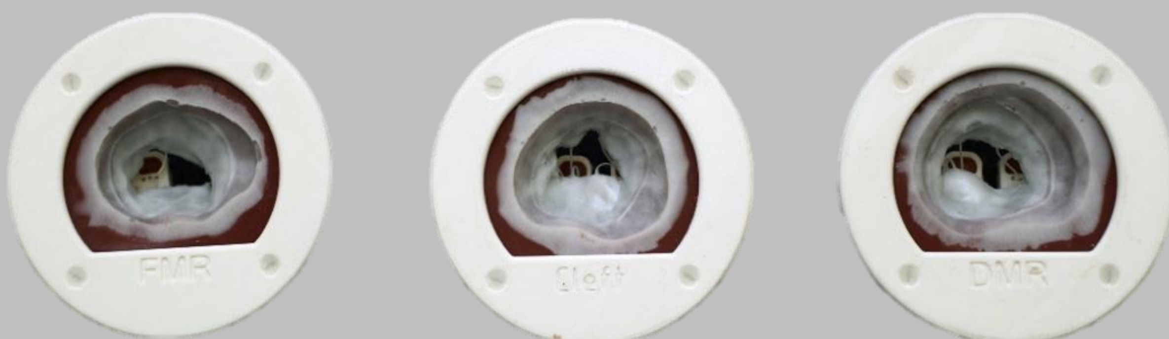
Figure 1: Interchangeable mitral valve apparatus designed for simulator, (functional mitral regurgitation, left; cleft case, middle; degenerative prolapse, right).
