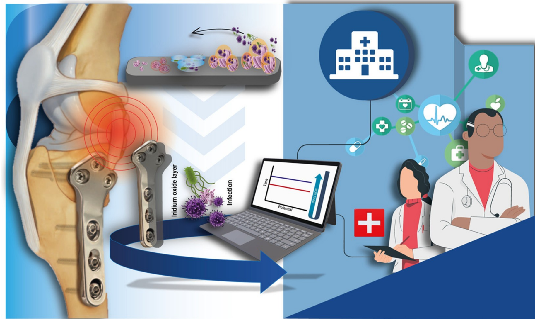
Concept: a titanium fixation implant functionalized with iridium oxide detects peri-implant acidification.
