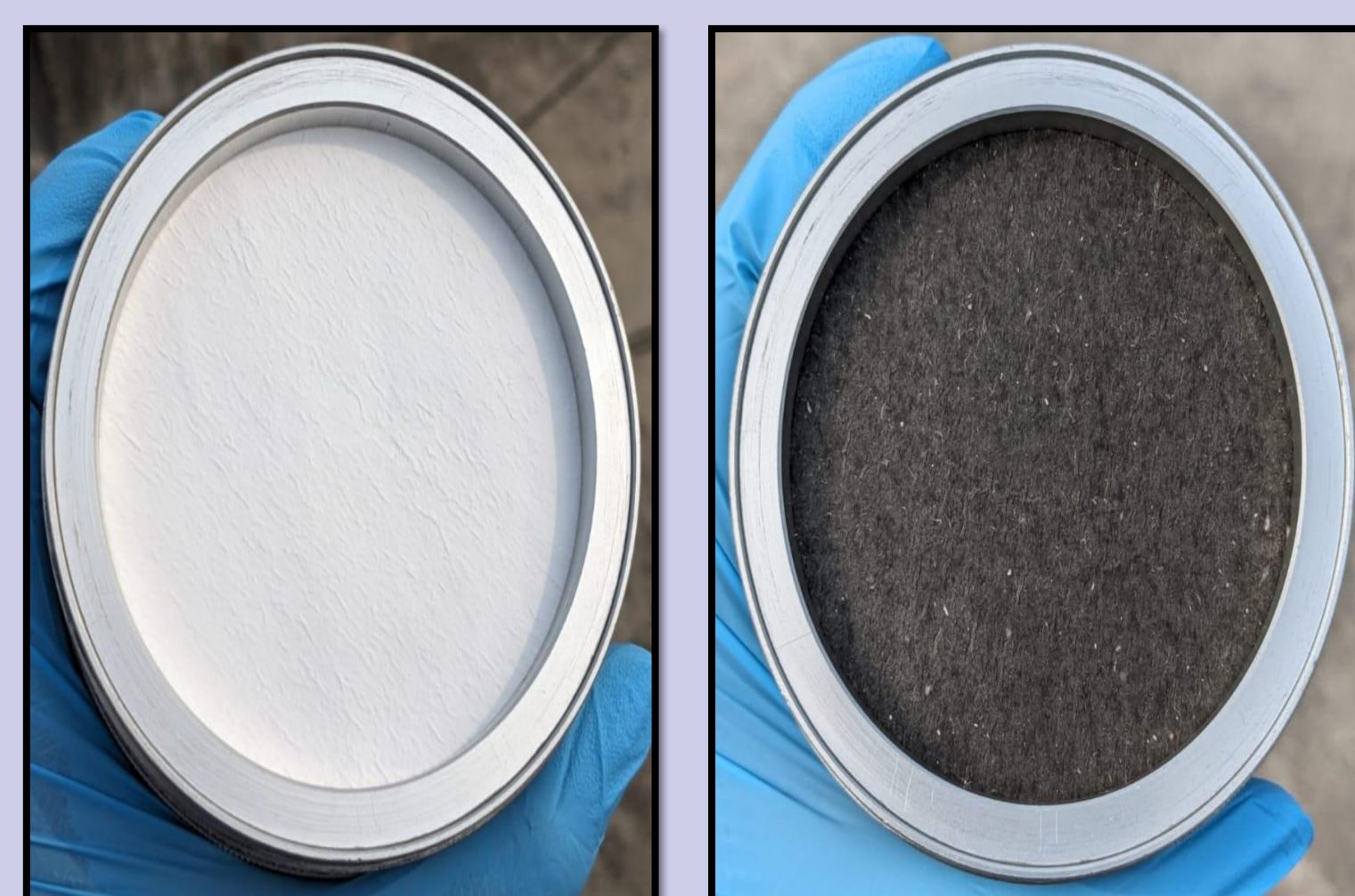
Figure: Quartz filter (a) before sampling (b) after sampling
