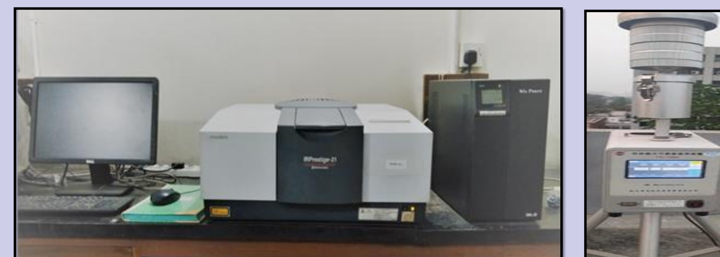
Figure: Used instruments in the study: (a) Fourier transform infrared (FTIR) spectrophotometer (b) TH-150H air sampler
