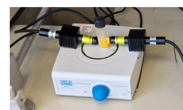
Fig. 4 Schematic illustration of the experimental setup of the photocatalytic degradation of PFOS using CIS and the corresponding PFOS removal% and defluorination%.
