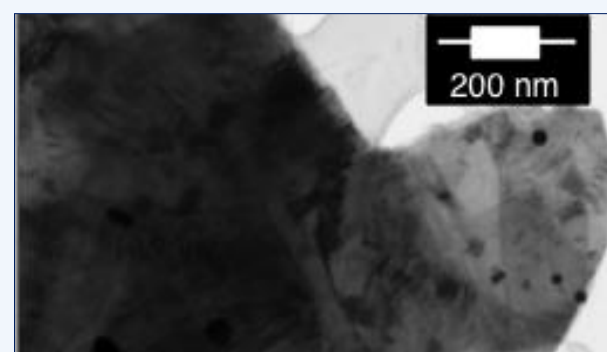
TEM of Supported AuNP on metal oxide Ave. size ~ 15-17 nm
