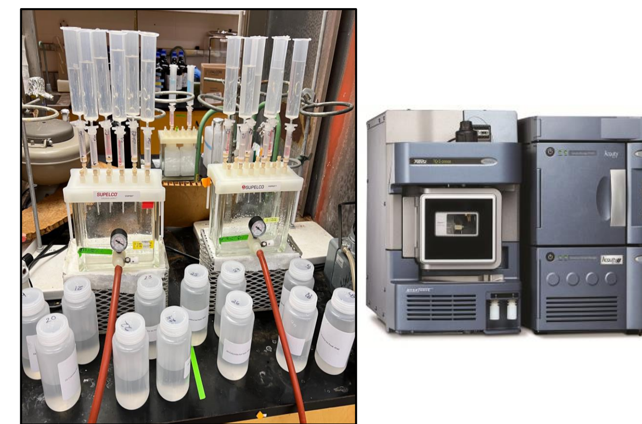
All samples were concentrated using SPE using Oasis WAX cartridges. Analysis was done using LC-MS/MS.
