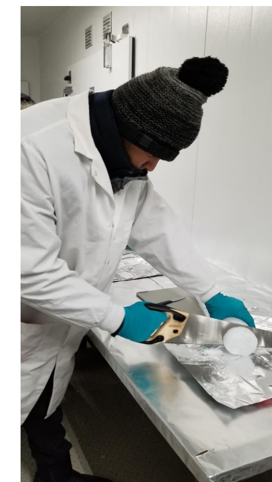
Ice core was sectioned into annual years using MeOH rinsed tools.
