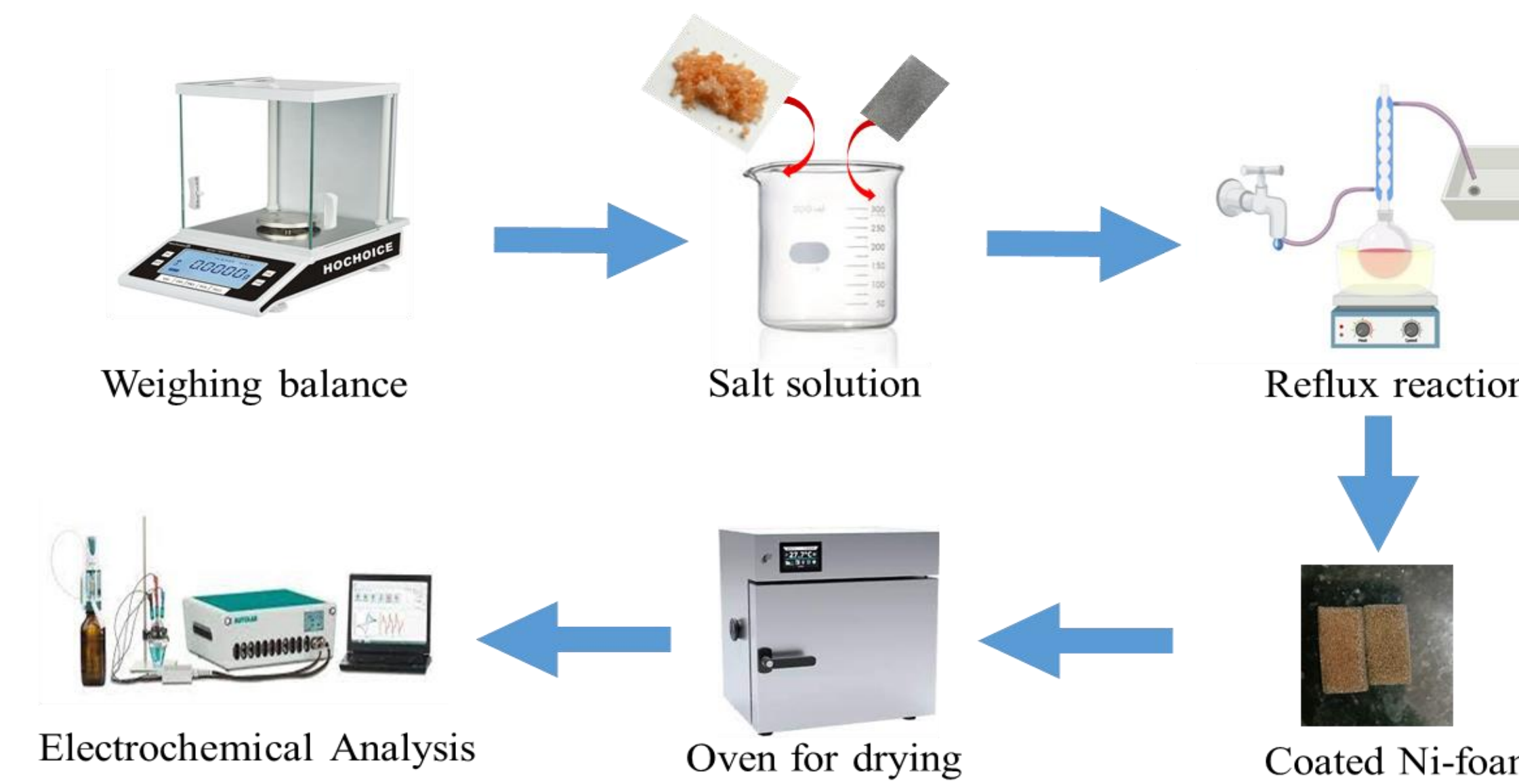
Figure 1: Systematic diagram for preparation of NiFe/NF via reflux method
