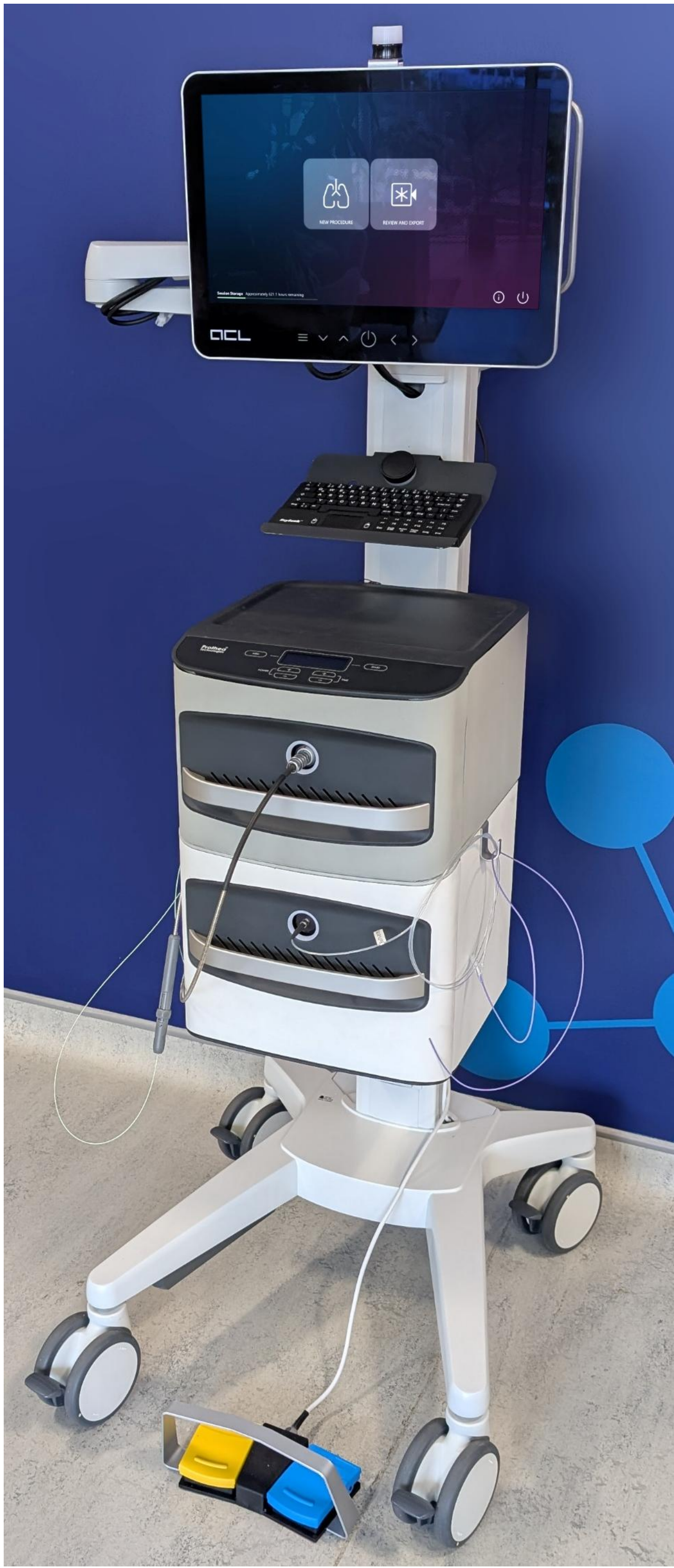
Figure 3. Our next-generation fibre-based FLIM system, namely KronoScan.
