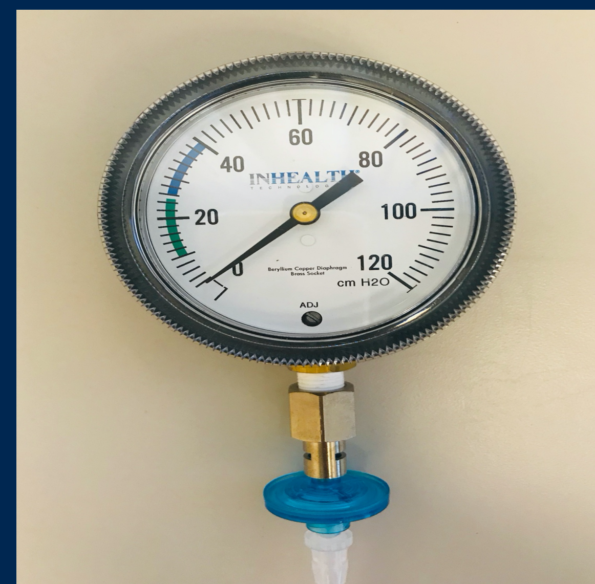
Fig 1. Blom-Singer intratracheal manometer
