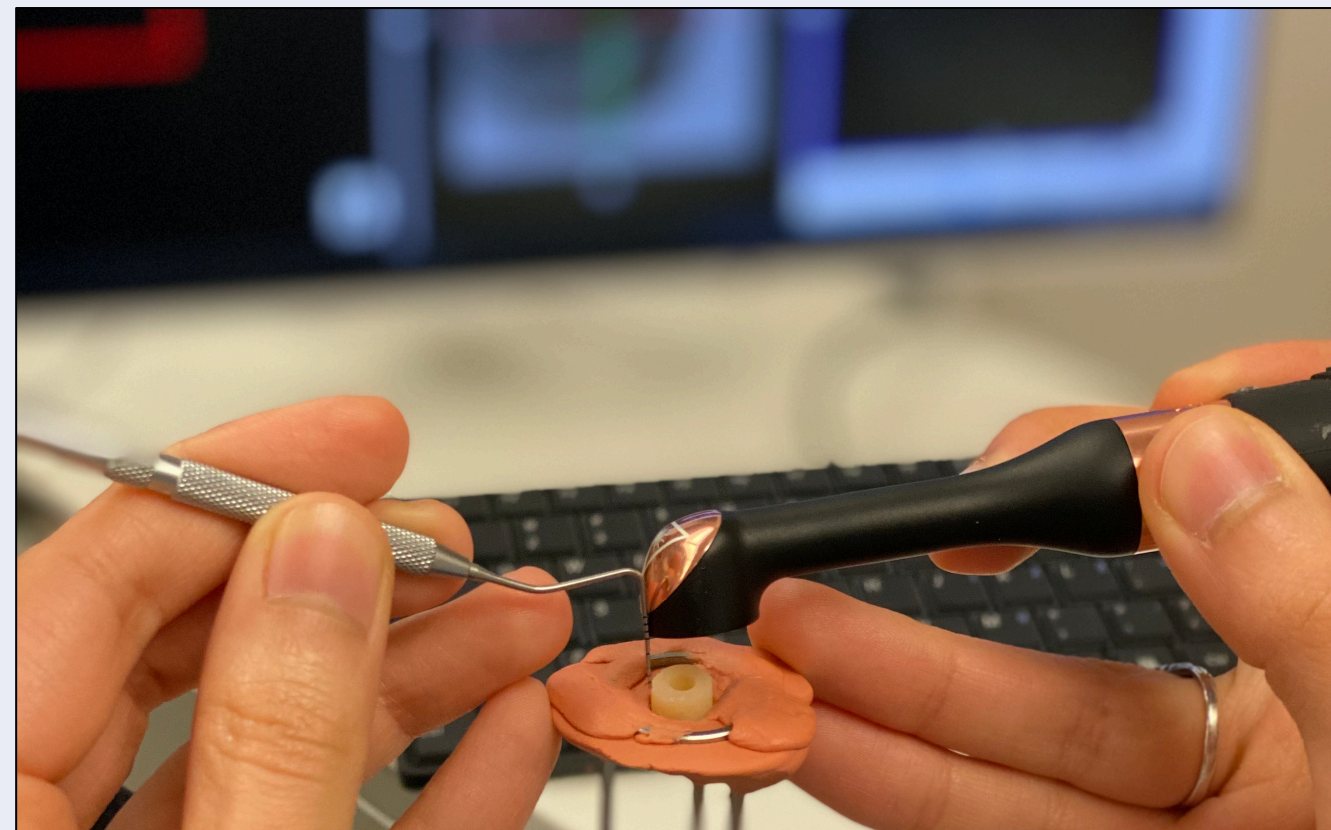
Figure 7 – Light curing unit at 8 mm distance from composite surface. Periodontal probe used for accurate measurement.
