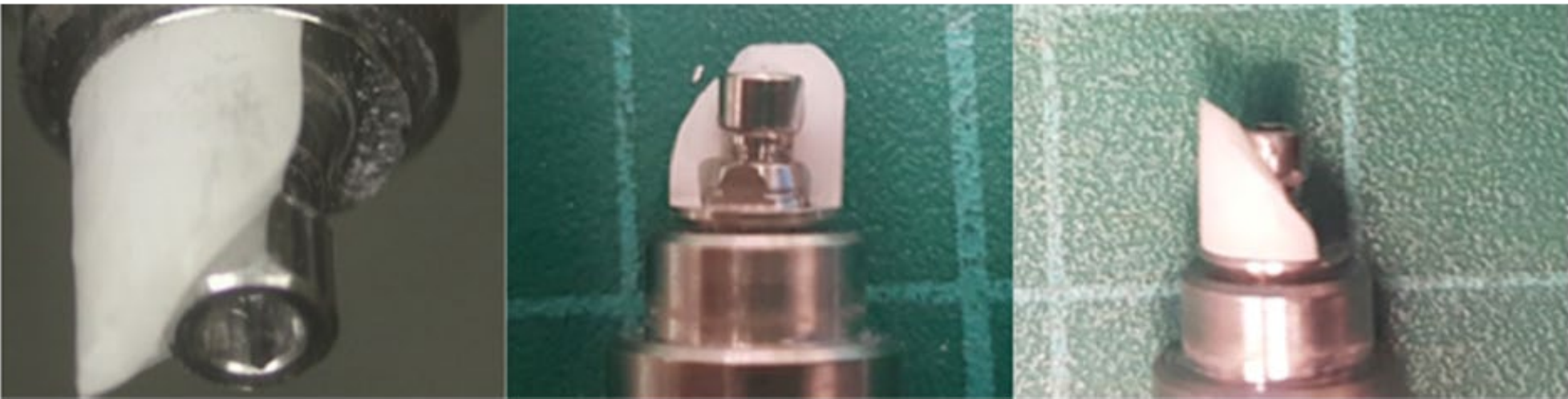
Figure 3. Specimen number one in group A shows fracturing of the zirconia concomitantly with bending of the restoration screw head under an applied load of 450 N. This failure was observed in group A at only high loading forces.
