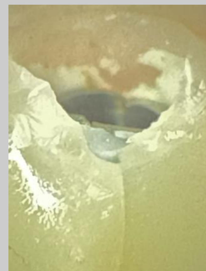
Fig. 3A - Fracture site with crack line along the zirconia
