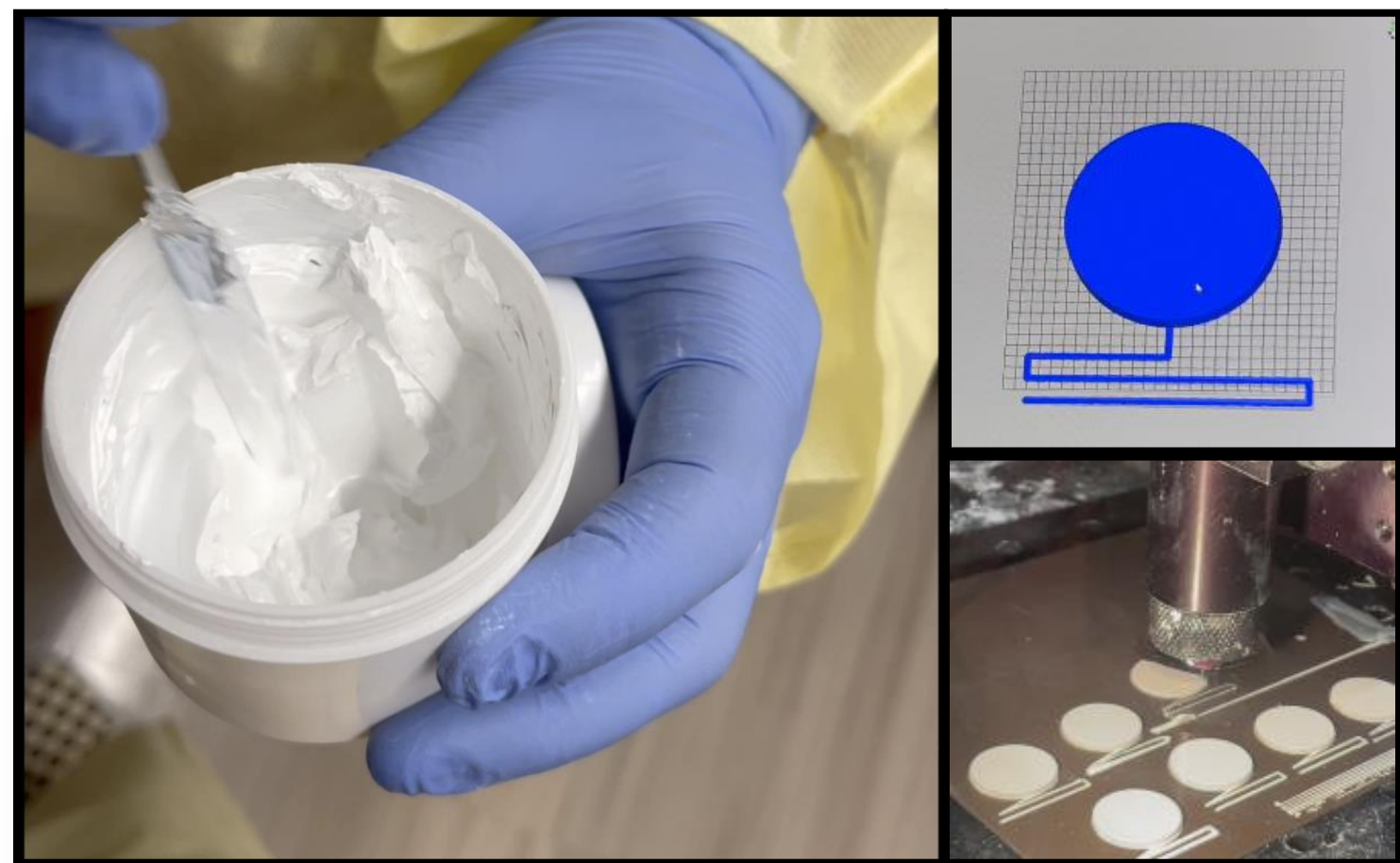
Figure 1. ATZ ink synthesis and 3D printing via direct ink printing, robocasting.
