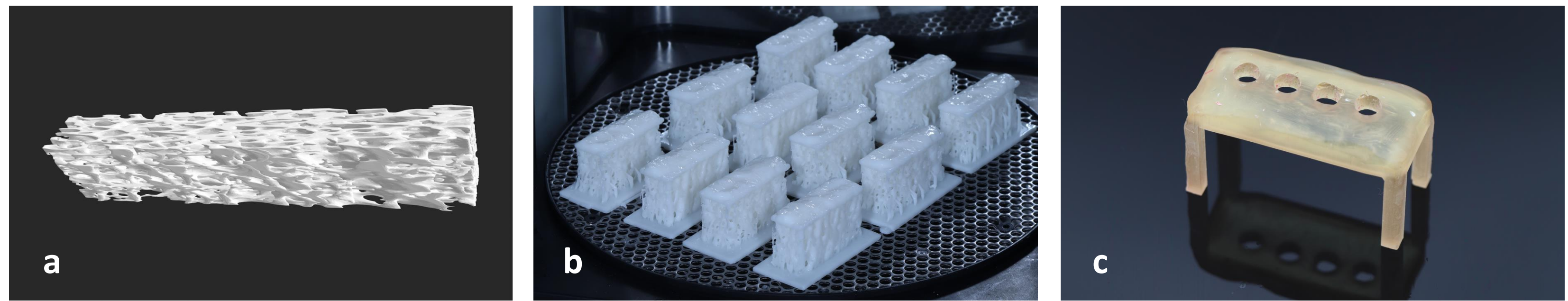
Figure 1: (a) STL of maxillary bone; (b) 3D printed bone models ; (c) 3D Printed Surgical Guide
