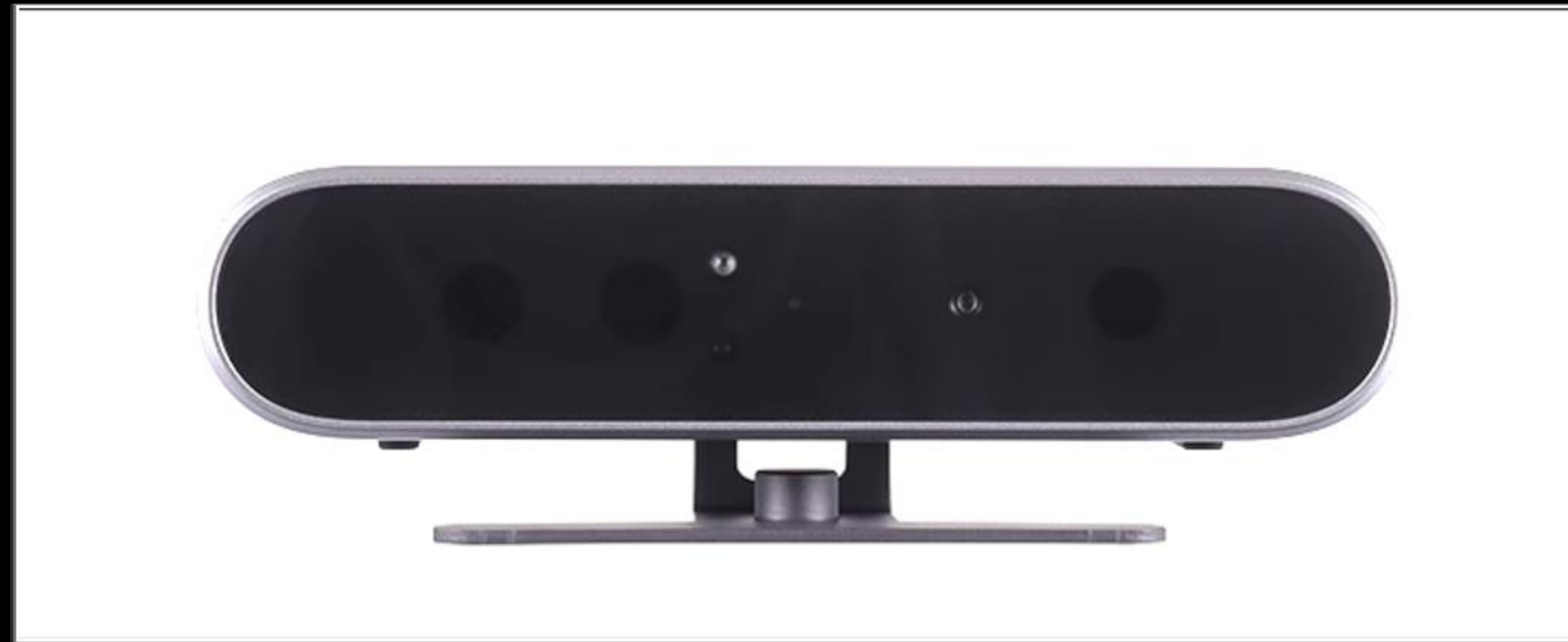
Figure 2: Component of markerless stereo vision system
