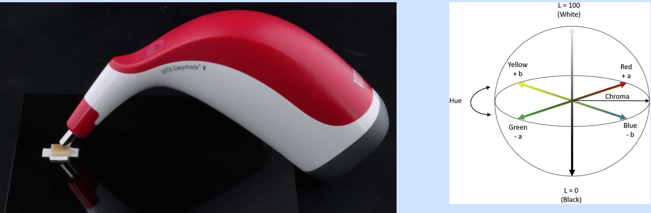
Figure 2: Shade coordinates (CIELAB color space) were measured with a spectrophotometer. The CIELAB color space expresses color as three values: L* for perceptual lightness and a* and b* for the four unique colors of human vision: red, green, blue and yellow. 2
