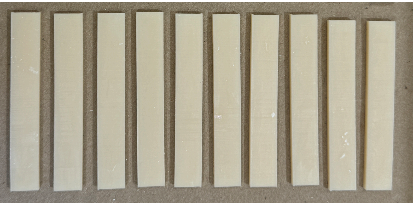
Samples from Straumann Printer (64mm x 10mm x 3mm)
