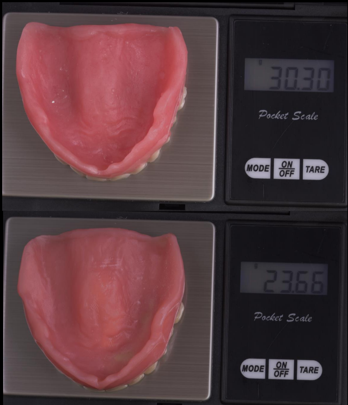
Fig 9) Conventional denture (top) weight and 3D Printed hollow denture (bottom) weight
