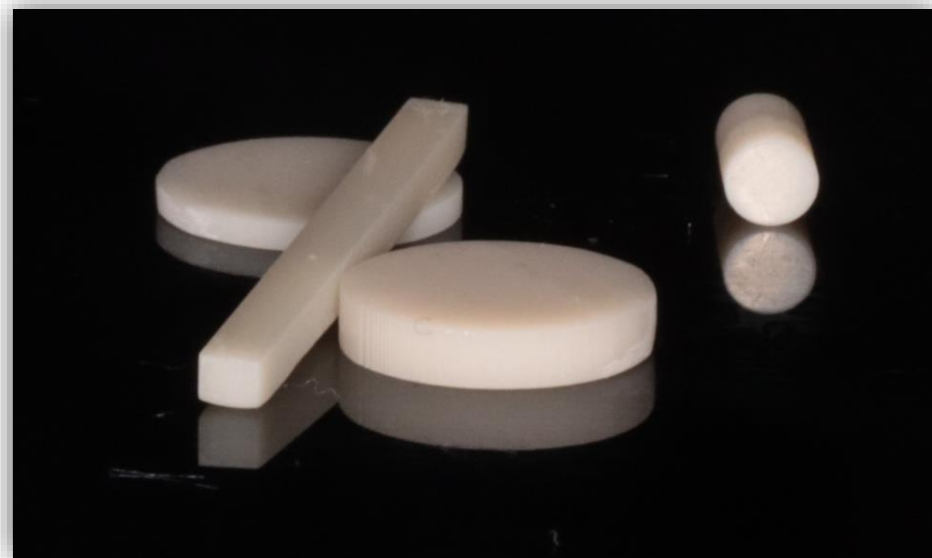
Figure 2: Specimens were prepared using a DLP printer, a 5-Axis open technology system milling machine, and Teflon molds.
