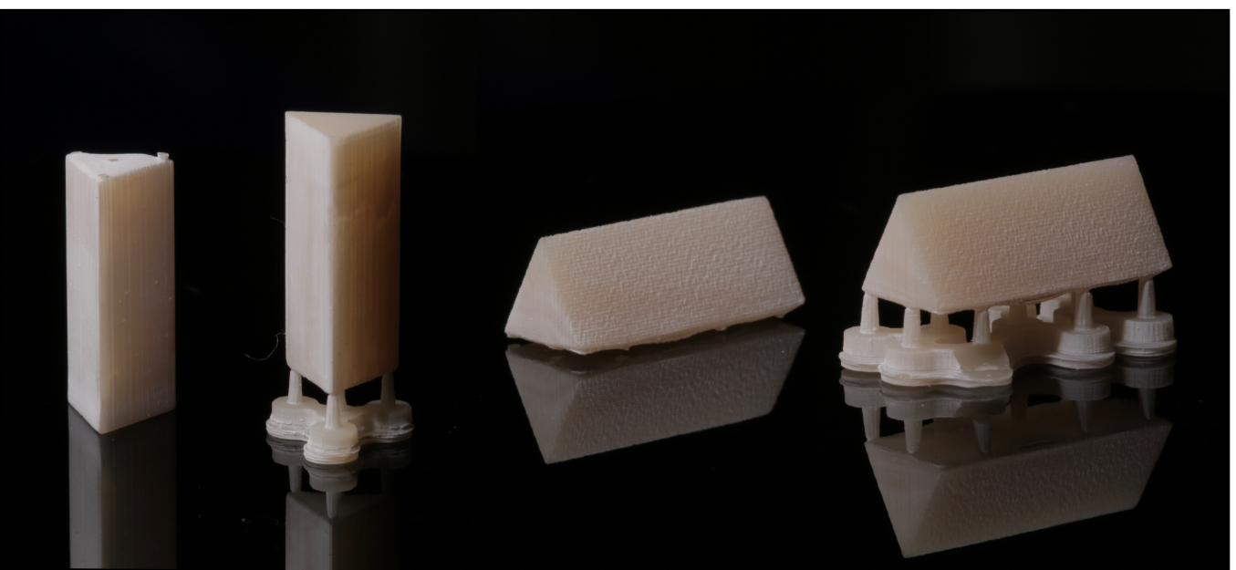
Figure 2: NTP 3D printed specimens without and with supports (left prisms at a 90° print orientation, right prisms at a 0° print orientation).
