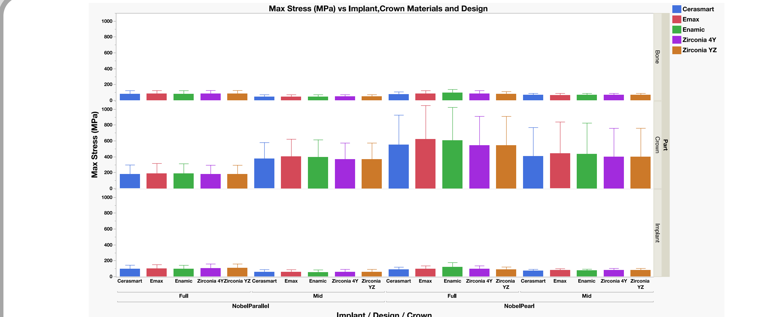
Fig:1 Max stress (MPa)Vs implant, crown Materials and Design
