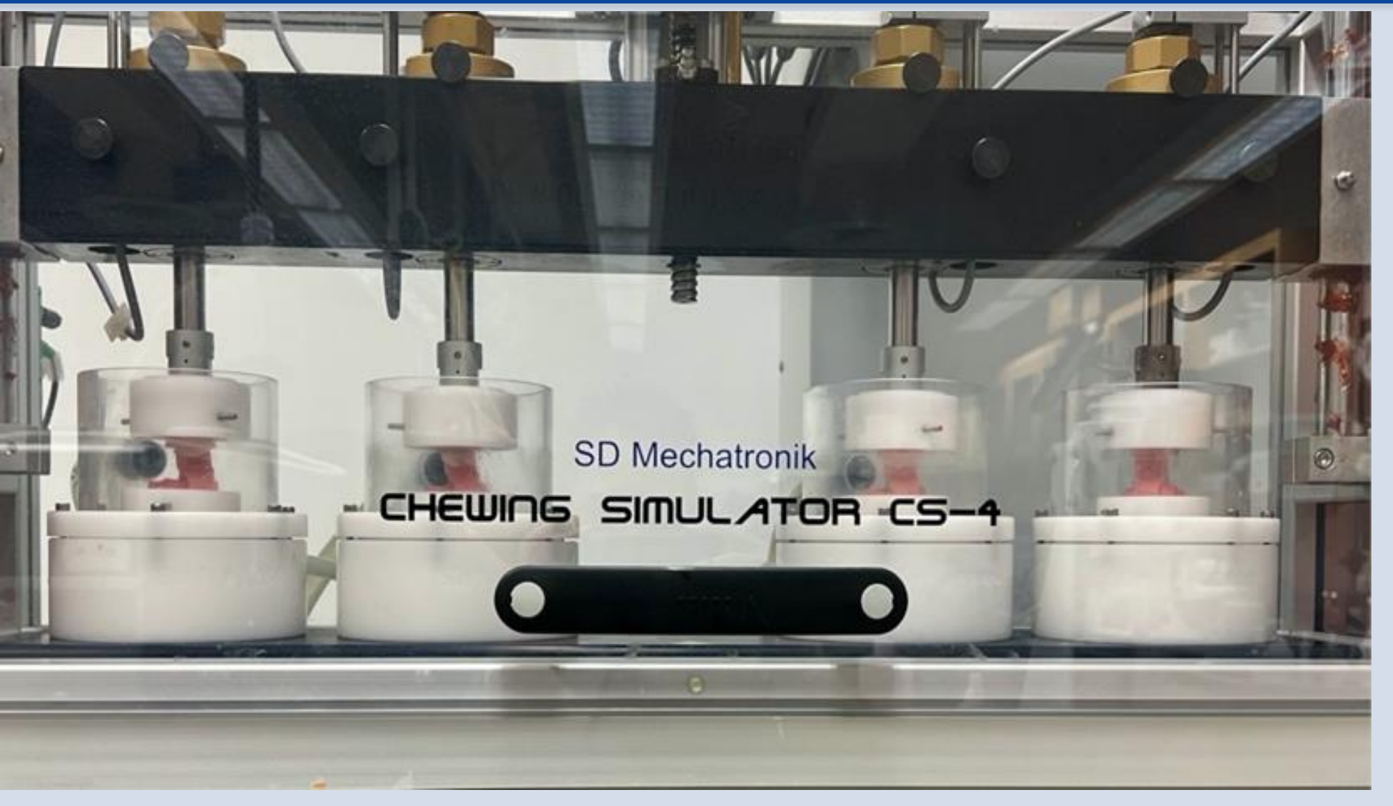
Fig. 6: Specimen were mounted in a chewing simulator machine (Chewing Simulator CS-4; SD-Mechatronik, Westerham, Germany) for two rounds of 120,000 cycles (equivalent to 6 month of chewing) under a loading force of 49 N at a frequency of 1.3 Hz immersed in 37°C running deionized water. The retention of the denture base was assessed after each 120,000 cycles. A digital stereo microscope at 30x magnification (Dinolite) was used to assess the nylon inserts after fatigue loading.
