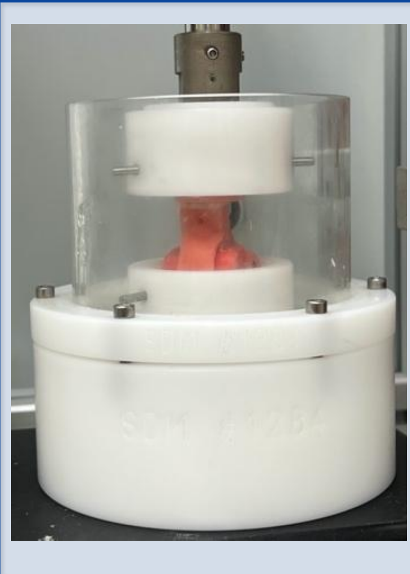
Fig. 6: Specimen were mounted in a chewing simulator machine (Chewing Simulator CS-4; SD-Mechatronik, Westerham, Germany) for two rounds of 120,000 cycles (equivalent to 6 month of chewing) under a loading force of 49 N at a frequency of 1.3 Hz immersed in 37°C running deionized water. The retention of the denture base was assessed after each 120,000 cycles. A digital stereo microscope at 30x magnification (Dinolite) was used to assess the nylon inserts after fatigue loading.
