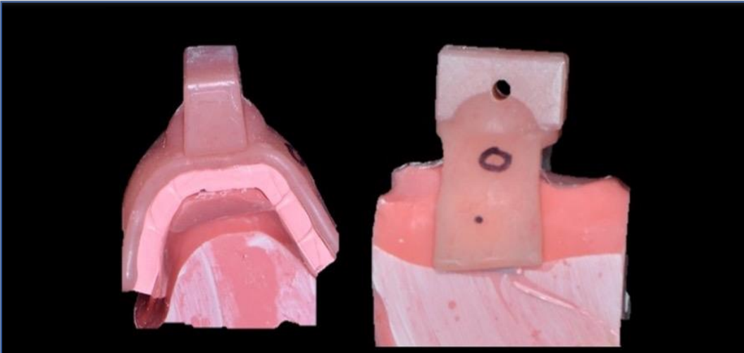
Fig. 4: Denture base was perforated to insert wire rope for the retention test.
