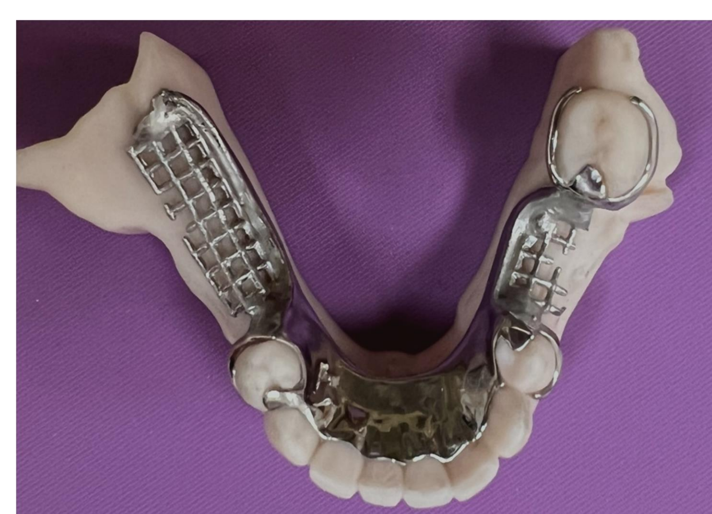
Fig. 5 Metal framework from printed wax pattern
