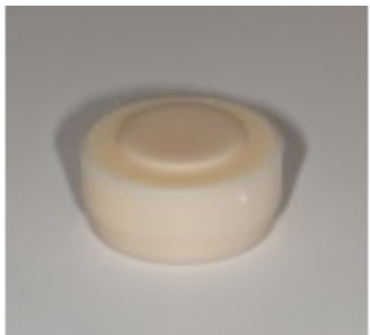
Fig. 1 Each disc was placed on a die with shade ND3
