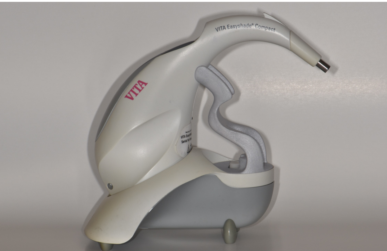
Fig. 3 Vita EasyShade Spectrophotometer, Preset Control and \Delta E measurements
