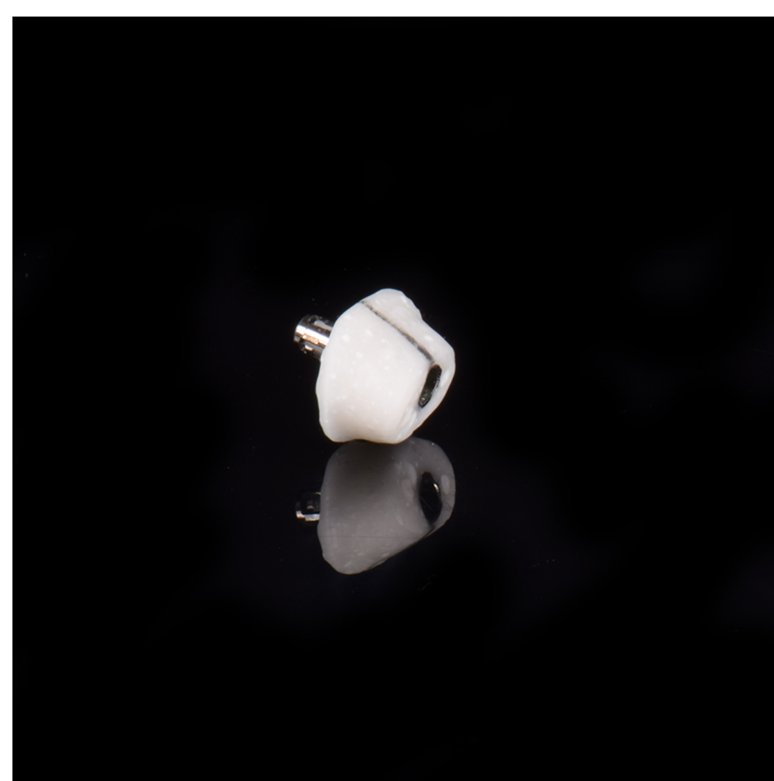
50/50 mix of barium sulphate and clear resin, prepared into cones with finish line and flat occlusal surface
