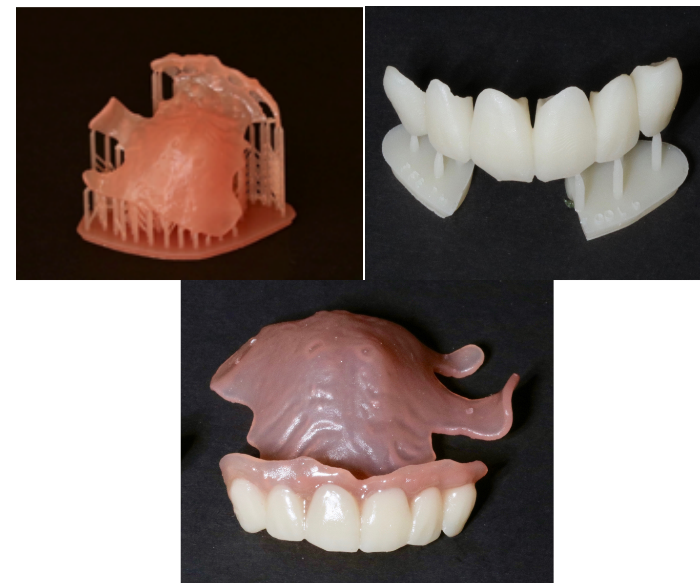
Fig. 4 Separately printed base and teeth. The base and teeth luted together.
