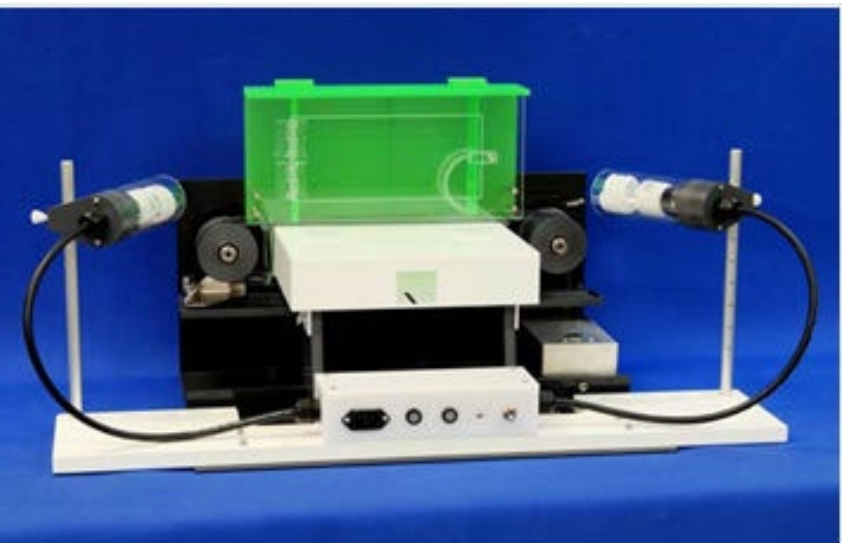
Figure 5. TreadScan apparatus. The mouse walks on a treadmill in a chamber illuminated by green light. A camera records data.
